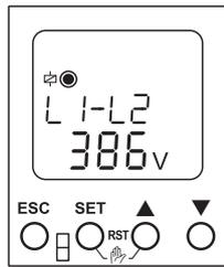
Display L1- L2 if work normally; display faults symbol when faults occurred.
